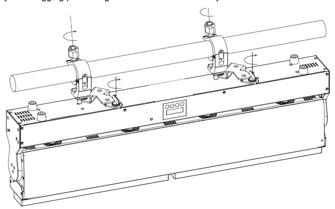
Regardless of the rigging option you choose for your LED pixel Zoom par, always be sure to secure your fixture with a safety cable. The fixture provides a built-in rigging point for a safety cable on the hanging bracket as illustrated above. Be sure to only use the designated rigging point for the safety cable and never secure a safety cable to a carrying handle.
